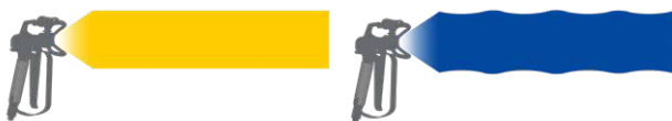
Fig.: At low pressure: even spray jet from the diaphragm pump (yellow) and irregular spray jet from the piston pump (blue).
